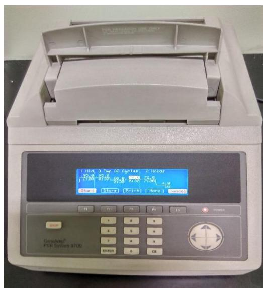
Slika 4.6. Uređaj GenAmp System 9700 (Applied Biosystems, SAD).
