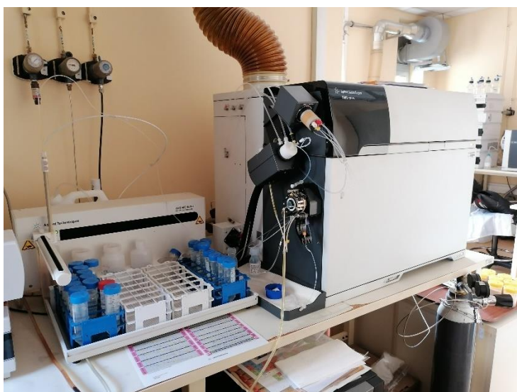
Slika 8. ICP-MS, Agilent ICP-MS system Model 7900 (Agilent, Palo Alto, CA, SAD).
